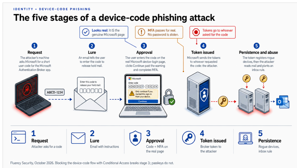
Figure 1. The five stages of a device-code phishing attack: request, lure, approval, token issued, persistence and abuse. Unlike AiTM, every page the victim sees is genuine.
